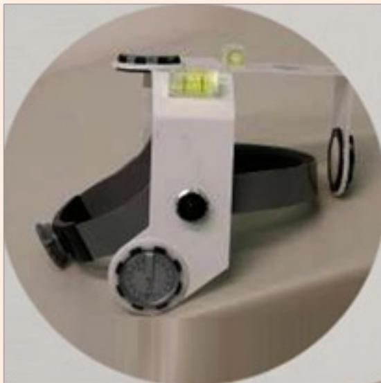
Figure 2: Analogic inclinometer.
